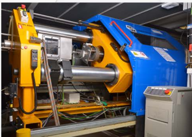
MWH's bespoke valve wear test rig with integrated environmental chamber simulates valve closure and peak firing pressure up to 900°C
